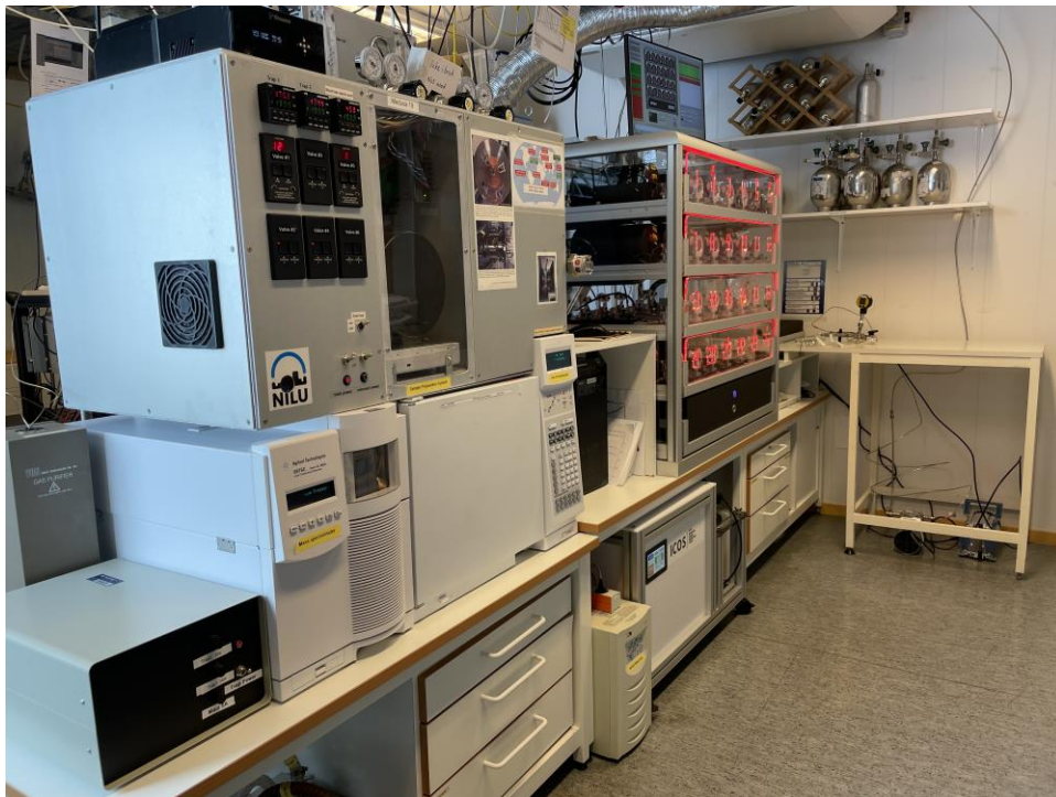
Zeppelin Medusa-GCMS next to ICOS flask sampler
